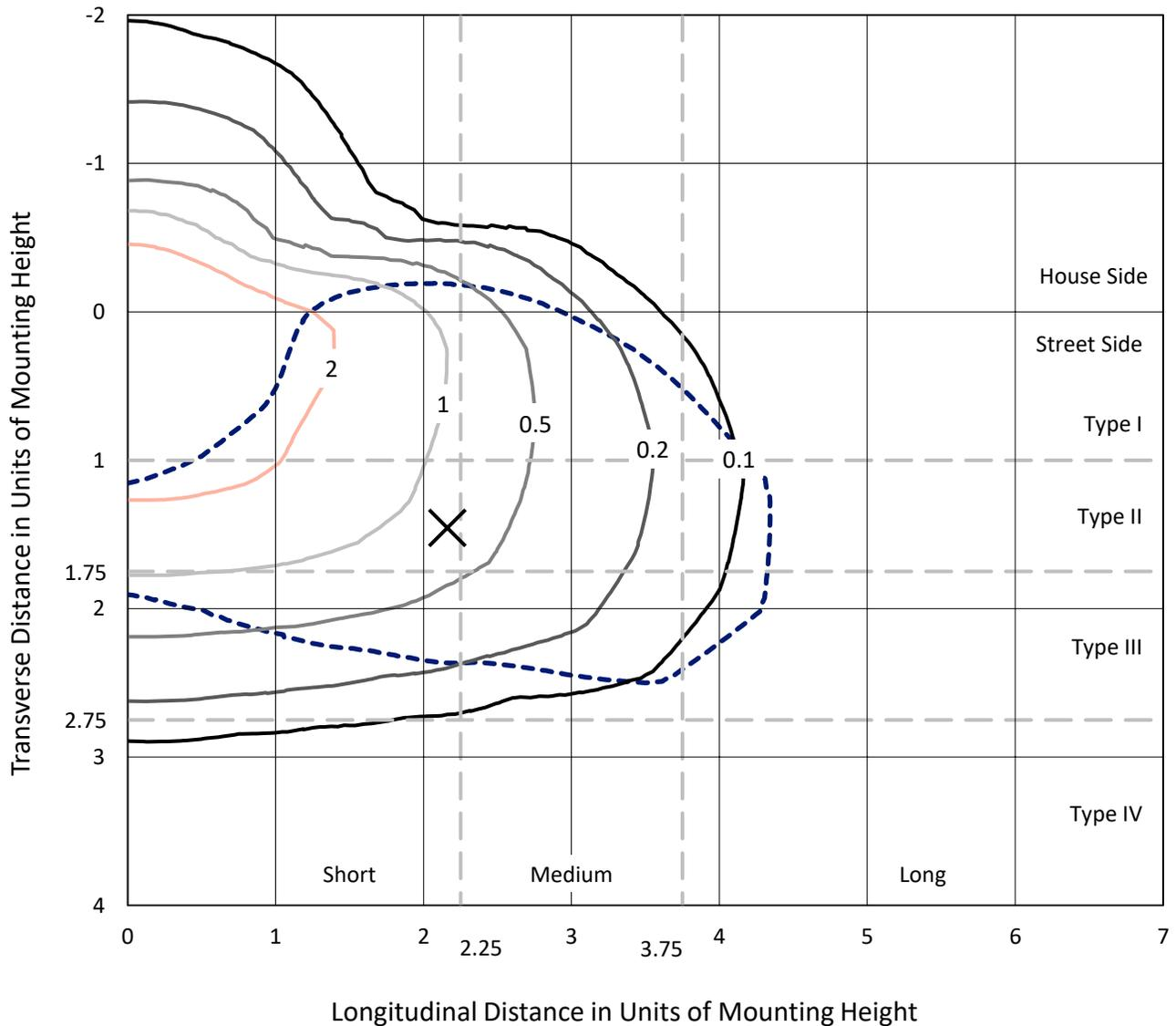
Based on 25 foot mounting height. Maximum calculated value = 3.7 fc
