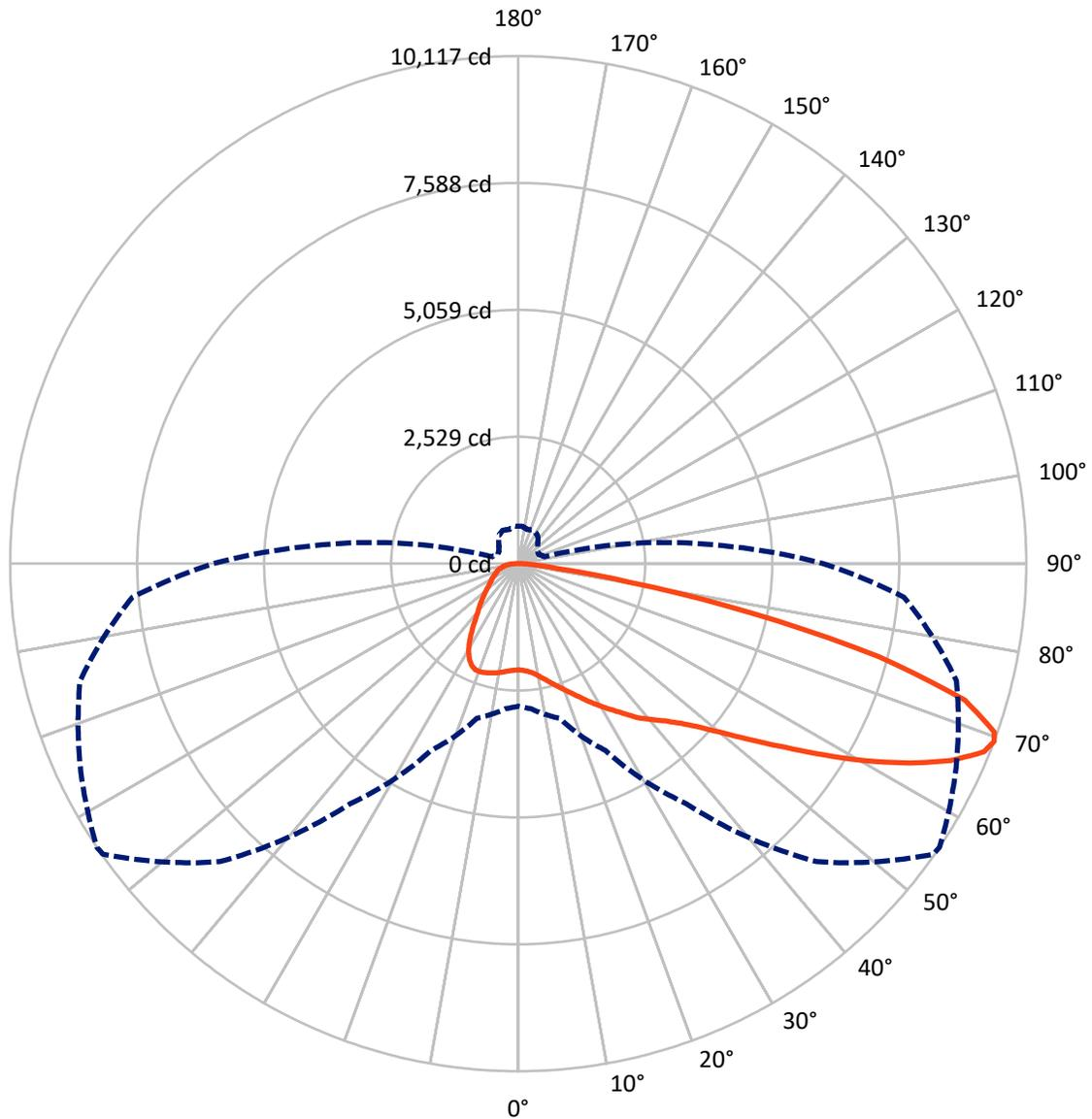
— Vertical Plane Through 56-Deg Lateral    - - - Horizontal Cone Through 69-Deg Vertical
